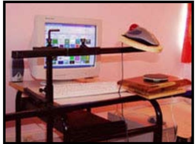
Our custom made trackball mouse stand. It can move in 3D and be positioned for any child. It enables children who cannot use a normal mouse to work on the computer.
